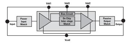
Single control bias setting for low Idq and 40%PAE at Pout = 28.5 dBm
